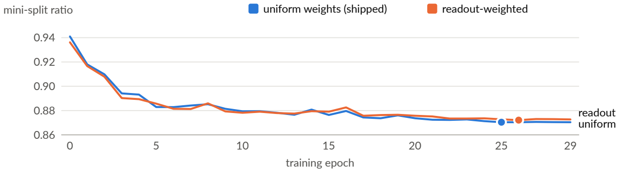
Figure 6. Ratio on the public mini split (corrected / uncorrected raw MSE) after each training epoch for the two loss weightings. Markers are the selected epochs. Each epoch took about 270 s on one L4 GPU.
